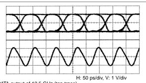
DATA output of 12.5 GHz (top trace) CLOCK 1 output (bottom trace)
